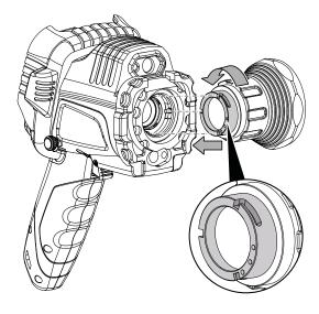
2. Rotate the lens clockwise until it is firmly attached to the camera head.
