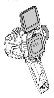
2. Open the protective cap at the IR lens (10).
