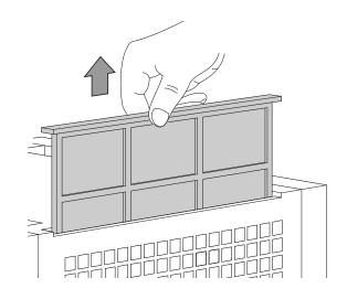
2. Clean the filter using a slightly damp, soft, lint-free cloth. If the filter is heavily contaminated, clean it with warm water mixed with a neutral cleaning agent.
